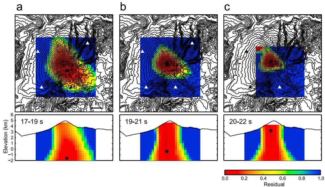
**Figure 3.** Horizontal and vertical distributions of the normalized residuals estimated for the explosion event in three time periods (17–19, 19–21, and 20–22 s) at the event onset. Stars indicate the minimum residual points. Dots indicate the nodes used in the grid search to estimate the source location.
