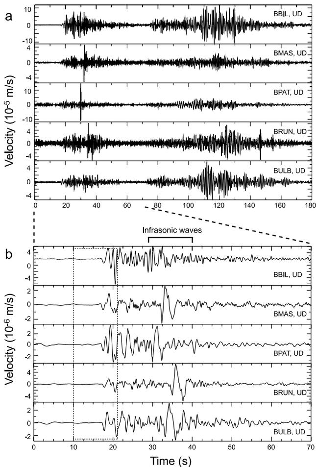
**Figure 2.** (a) Broadband vertical velocity seismograms of the explosion event at Tungurahua. The time axis in seconds is measured from 00:55 on 11 February 2010 (UTC). (b) Waveforms of Figure 2a band-passed between 2.5 and 10 s in a time period between 0 and 70 s. Signals enclosed by the dotted rectangle were used in the waveform inversion. The horizontal bar indicates seismic waves that were affected by infrasonic waves.
