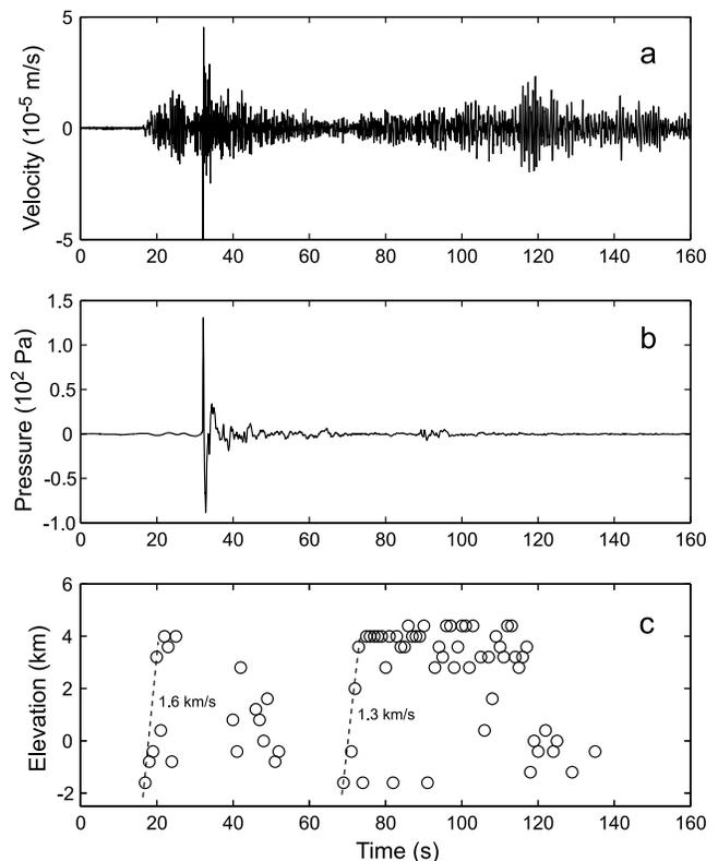
**Figure 4.** (a) Broadband vertical seismogram, (b) infrasonic waveform observed at station BMAS, and (c) source depths estimated from high-frequency seismograms plotted as a function of time.
